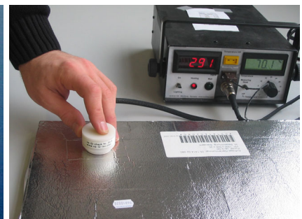
Check of the gas pressure in the panel
