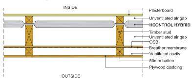
In walls once installed, the R Value of HCONTROL HYBRID with adjacent air cavities was measured at **3,45** m².K/W, slightly over the laboratory measured R-value.
