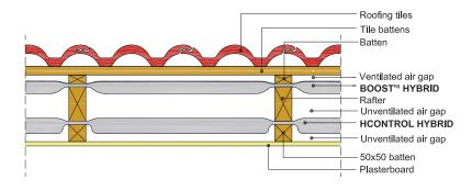
In roofs once installed: The R Value of BOOST'R HYBRID with adjacent air cavities was measured at **2,17 m².K/W.**The slight difference from the performance in a laboratory is due to the fact that BOOST'R HYBRID has been measured with a ventilated air gap on the cold side, which is not taken into account in the laboratory tests.
